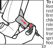
lbs. (10.1-18 kg), 34-43" (85.1-110 cm), Over 1 year of To remove LATCH: Remove child from child age restraint. Press down firmly on adjuster side of child restraint and press release button to release tension. Unhook LATCH from bar by squeezing spring lever and twist hook.
